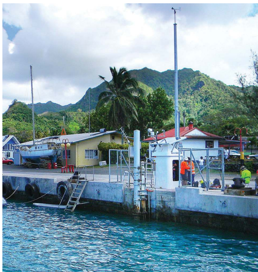
Figure 4. Technicians working on the Cook Islands tide gauge, which has been monitoring sea level and weather conditions in Rarotonga for over 25 years. Photo: Stamy Criticos (2012).
